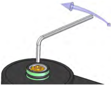
Figure 9 Adjusting flow rate.
