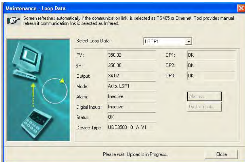
Figure 4-12 Loop Data Maintenance Screen
