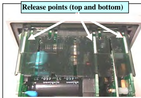
Figure 3 Removing Printed Circuit Boards
