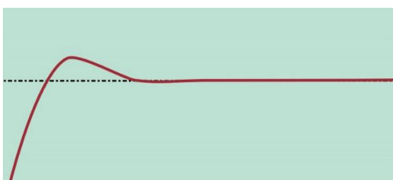
Too Small: Overshoots setpoint before settling
