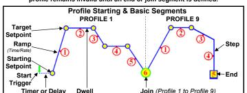
Timer or Delay Dwell ollowing a Start Trigger, profiles can start immediately, or if enabled after a delay or at a specified day & time (Recorder only).
