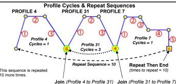
profile can be made to run itself 1 to 9999 times or continuously using the Profile ycles setting. A profile ending with Repeat Then End will run the entire sequence of profiles again 1 to 9999 times or continuously.
