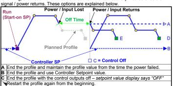
On Recorder versions, option E will always be used if the power / signal is lost for less than the Profile Recovery Time. If the power / signal is lost for more than this time the defined Profile Recovery Method is used.
