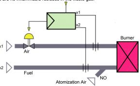
It is normal in this application to display the process value and setpoint as relative values rather than the physical ratio or absolute values. A scaling factor is set such that the displayed value will be 1.00 at the correct stoichiometric ratio for the
