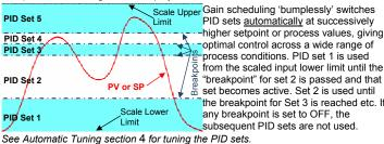
NOTE: ON/OFF control is possible with the individual PID sets but cannot be used with gain scheduling. On/off control is replaced with the default proportional band if gain scheduling is turned on.
