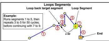
Loop Segment goes back to a specified segment. This action is repeated for the equired number of times (1 to 9999) before the profile continues onwards. More than one Loop Segment can be used, but they must not cross
