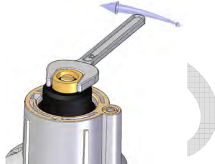
Figure 24: Adjusting flow rate.
