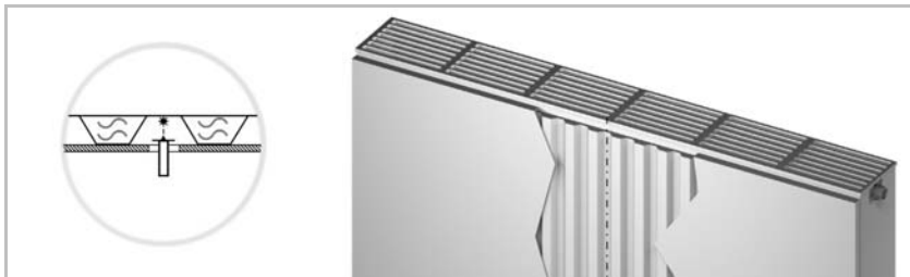
Determine the centre of the radiator length
