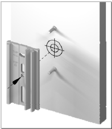
Welding position installation plate
